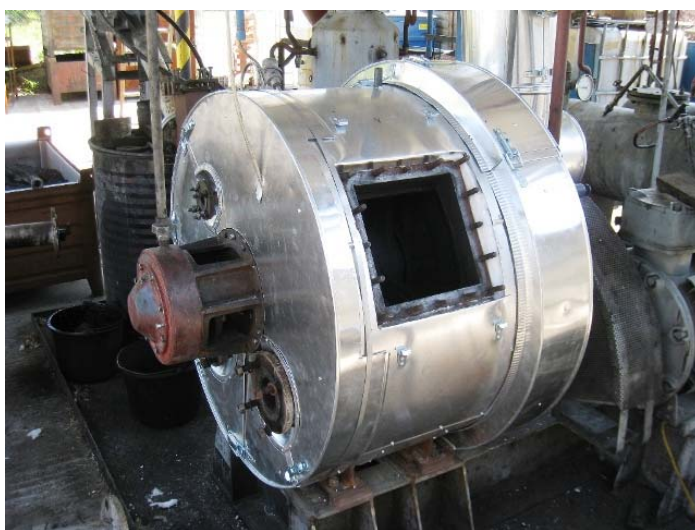
Picture 1 - 45 kW Blowdec reactor built in 2002 with maintenance opening
