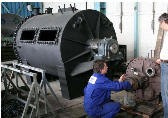
Picture 2 - 800 kW reactor built in 2007 with 2 maintenance openings (and 45 kW reactor in workshop)
