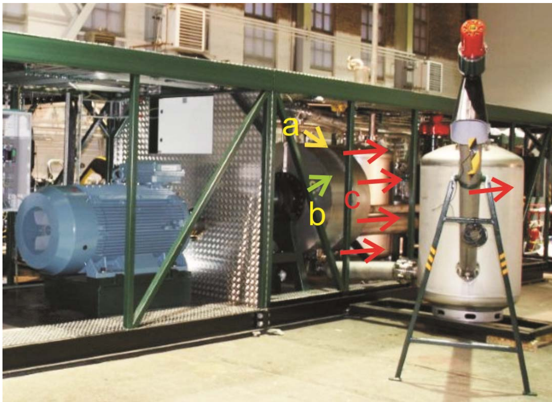
Picture 4 - 600 kW Cassandra Oil Reactor (source www.cassandraoil.com )
